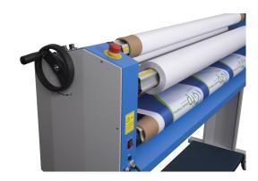
Integrated Rear Rewind makes Roll-to-Roll applications easy.
