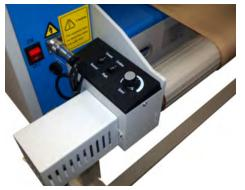
Motorized rear rewind for roll-to-roll applications
