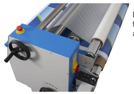
Motorized rear rewind for roll-to-roll applications
